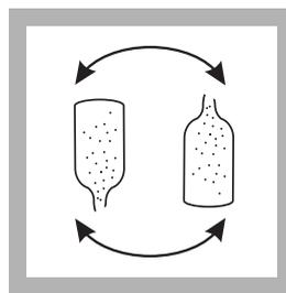
**7. Quickly invert the ampul several times to mix. Wipe off any liquid or fingerprints.**
