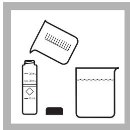
3. Fill a sample cell with at least 10 mL of sample (the blank). Collect at least 40 mL of sample in a 50-mL beaker.
