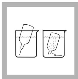
**6. Fill a Ferrous Iron AccuVac Ampul with sample.**
