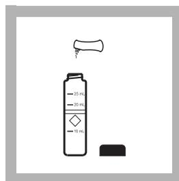
**7.** Add the contents of one Ferrous Iron Reagent Powder Pillow to the sample cell (the prepared sample). Cap and invert to mix.
