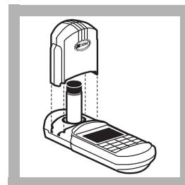
**4.** Place the blank into the cell holder. Tightly cover the sample cell with the instrument cap.
