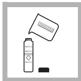
**3.** Fill a sample cell with 25 mL of sample (the blank).
